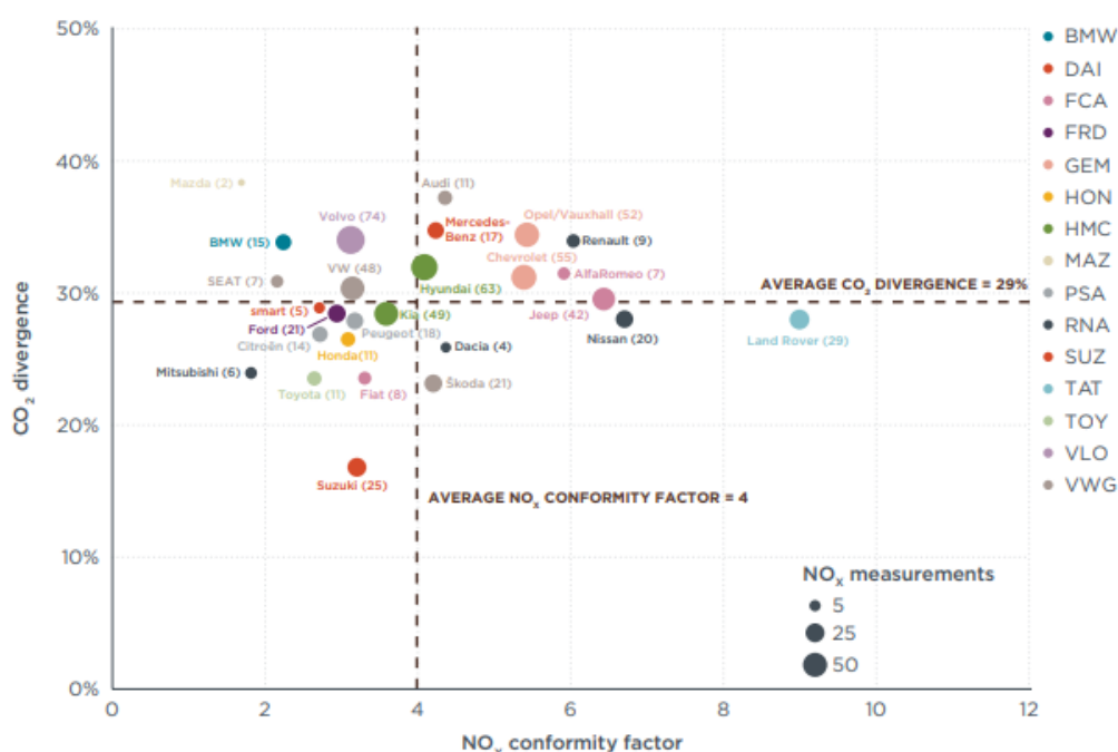
Figure ES-2: Euro 5 diesel passenger car gap between real-world and type-approval CO 2 emission values vs. on-road NO x emissions conformity factors by manufacturer. 3
